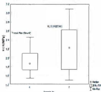
Fig. 5: Influence of type of hydraulic lime on bending strength (MOR): formula 4 and 7.
