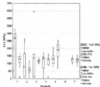
Fig. 1: The bending strength (MOR) of “wet” and “dry” specimens.
